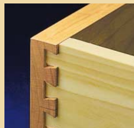
Too Deep. If pins go deep, move template forward. Too Shallow. If not deep enough, move back.
